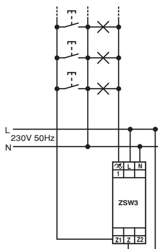
If a pulse relay in an existing installation is to be replaced by the ZSW 3 in 3-conductor circuit configuration, one of the potential-free central inputs can be used for this purpose. However, the load capacity of this input is limited to 1mA glow lamp current.
